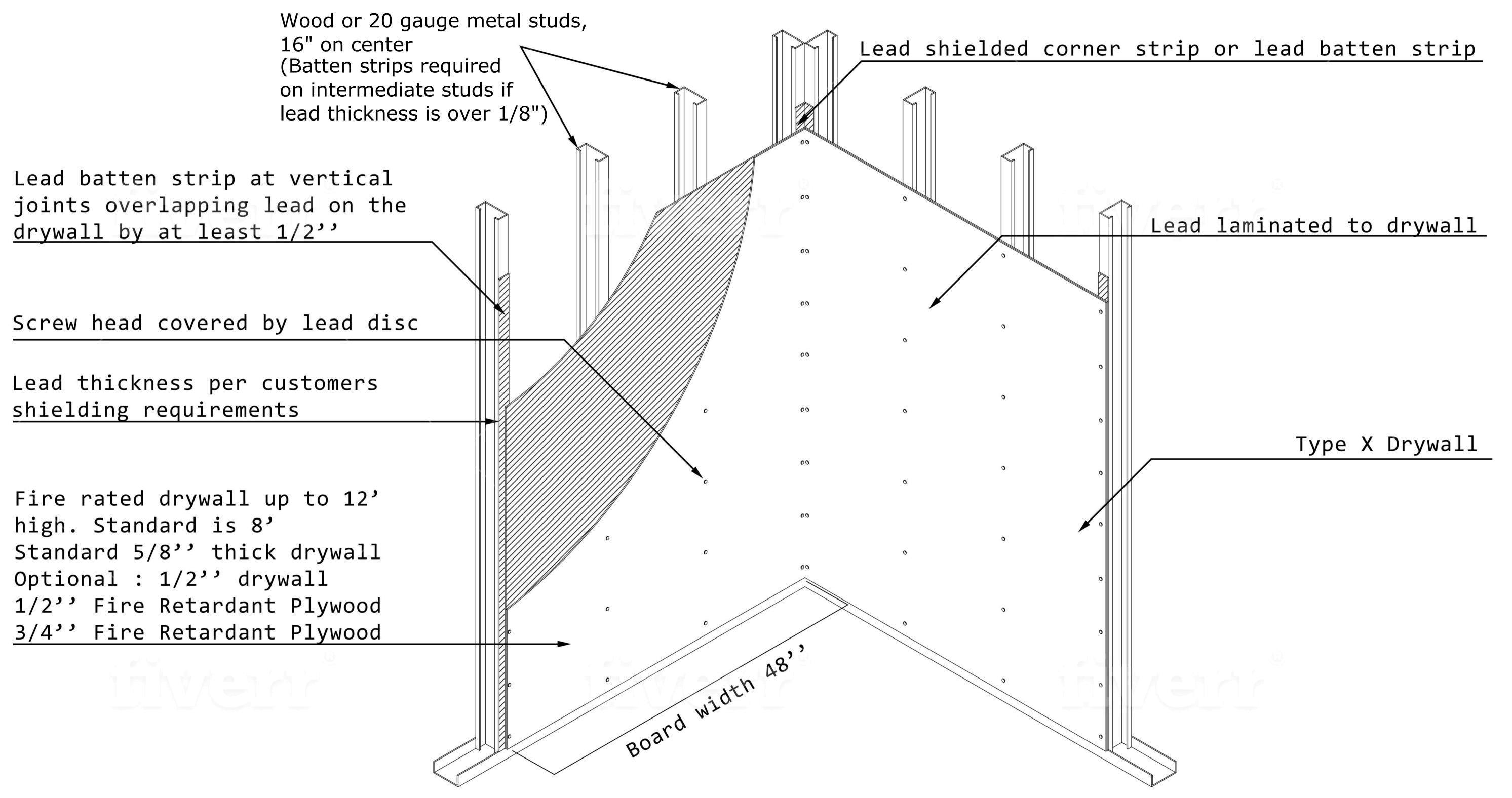
Screw layout: 8' on center of the vertical edges 12' on center at intermediate studs
